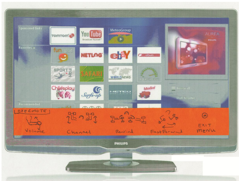
Figure 7 – The interface on the television screen would consist of a colored bar on the bottom to contrast against the background and would include blinking pictures of the exercises for each function.
